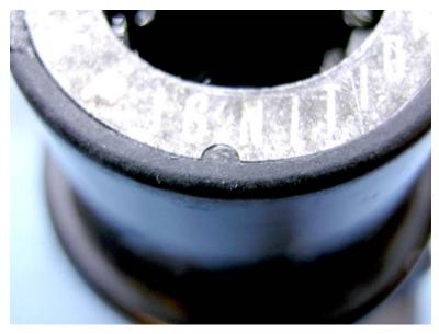
Now to put the decal back on. "But it won't stick anymore," you say. Nothing a bit of superglue can't fix... and you won't have to worry about positioning it the wrong way, because there's a little locating notch. Might not hurt to put a semi-heavy object on it for a minute or two so the glue has a chance to set.
