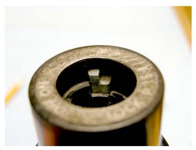
Normally, that piece sits like this, which keeps the lock plug from turning past the OFF position.
