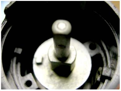
So where were we?... oh, yes. The lock plug with the spring, and this piece on top of the spring. Don't forget to smear some grease along the bottom surface (especially that sloped edge).
