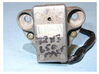
Here's the bottom of the switch module after it's been removed. Note the sticker – it's got the key code on it, should you need to have a replacement key made.
