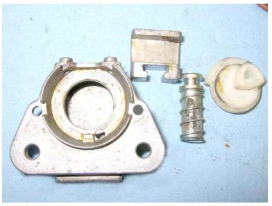
With your fingers holding in the top and bottom of the assembly, lift out the plastic piece. The backside has an offset triangular shaped cam. When you turn the key to the "LOCK" position, that cam pushes down on the spring-loaded pieces you see lurking in there. That makes the little stud stick out the bottom, which locks the forks in place.
