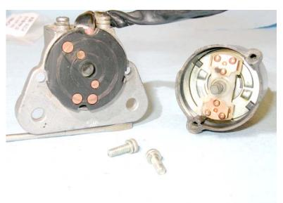
Insert the piece with the bumps on it – make sure the bumps face towards you. Don't forget to put a light coat of grease here as well. Next, add the plastic piece with the copper contacts. It should look like the part on the right when it's on.
