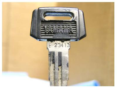
The key has a matching code. (We've used graphite to make the code easier to read.)
