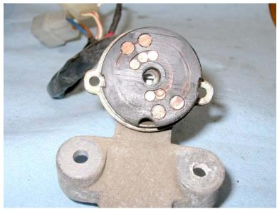
Extra wiring means extra copper pads on the contact plate.
