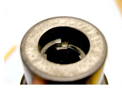
When you want to unlock the forks, you reinsert the key and turn to the ON position; the sloped edge on the bottom of that piece then pushes the slide back up into its normal position, and again blocks the key from turning past OFF.
