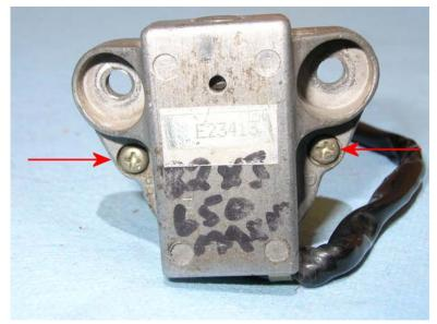
Let's break this puppy down. We start by unbolting the bottom section from the base. Remove the two screws shown and carefully separate the two sections.
