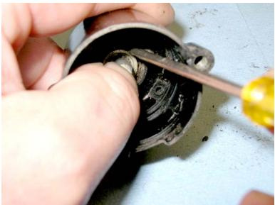
While doing that, press on the bottom of the shaft with your thumb. **S-L-O-W-L-Y**.
