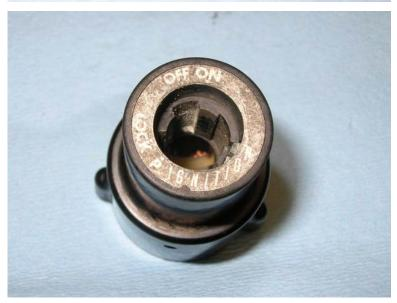
The protruding wafer(s) extend into the large slot at the top or bottom of the outer cylinder, depending on how the plug is installed. With the proper key inserted, the wafers retract, and allow the lock plug to rotate.
