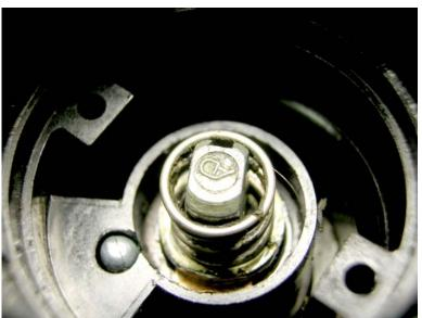
Once you've cleaned, lubed, and put that back together, it's time for final reassembly. Set the fork lock/contact assembly aside for now and reach for your lock cylinder.
