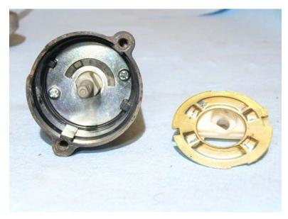
Now, the flat shiny piece with the slot. There are two locating cutouts on the edge. Lightly snug down the two screws (some housings are metal, especially the newer ones, but most of the original ones are plastic, so be careful not to crossthread).
