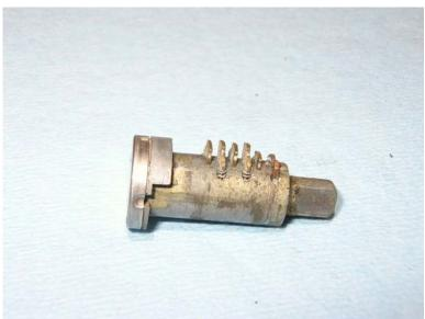
Before we go any further, let's go over the type of lock we're dealing with. A standard "pin tumbler" lock uses springs, driver pins, and key pins of various lengths inserted into a plug. The plug is inserted into an outer lock cylinder. Where the plug and cylinder meet is known as a "shear point". When no key or the wrong key is inserted, the point where the driver pins and key pins meet does not line up with the shear point, and the plug will not rotate.
