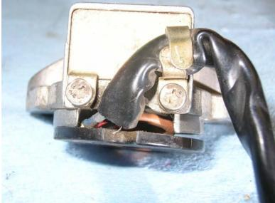
Now for the fork lock mechanism. Remove these two screws holding that metal retaining plate in place – the wires for the contact plate are loosely crimped onto it.
