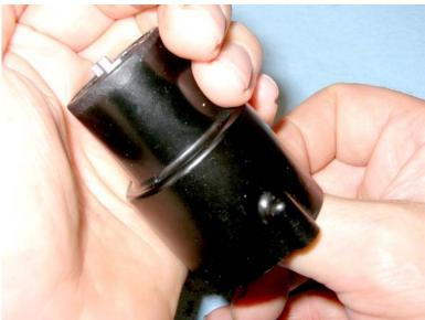
The next step is to push it out from the bottom using a thin tool or rod of some sort. Go slow, and cup the body in your hand. Why do this?
