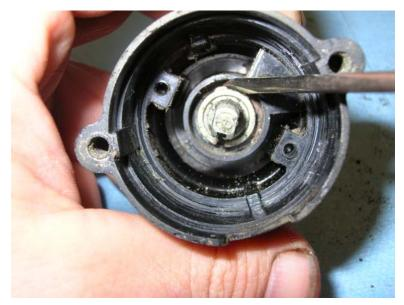
Since we have enough room, a small flat blade screwdriver will suffice to press the retaining latch/wafer inward.
