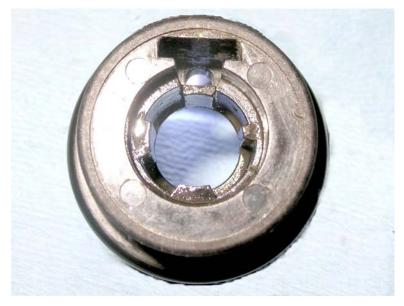
With the slide out, you can clean the slot it sits in. A q-tip might come in handy here. Then a light coat of grease on the slide, put the pin and spring back in the hole, and reinsert the slide into its home.
