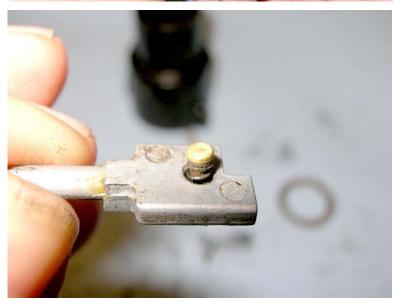
Right here – there's a spring-loaded pin that keeps it from sliding around at will. It's not as small as the wafer springs, but you don't want to have to go looking for this, either.
