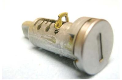
Reassembly, they say, is the reverse of removal. Spring in the hole, followed by its wafer.
