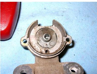
The plastic piece we saw earlier is metal here, and has a post on the back instead of a triangular cam.
