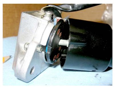
Finally, merge the two halves together and snug the screws down. Again, be careful not to crossthread the holes, especially if your housing is plastic (some are metal).
