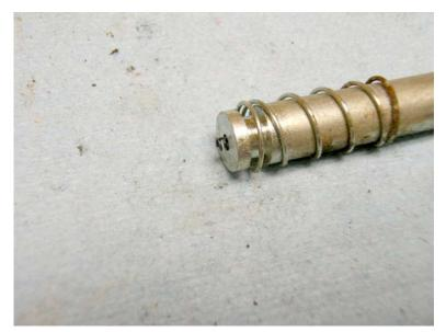
Here's the thing you really need to worry about – the post that sticks out and prevents the forks from turning has a weensy little spring in the top of it. This puts tension on the post and keeps it from flopping around in the piece that holds it.
