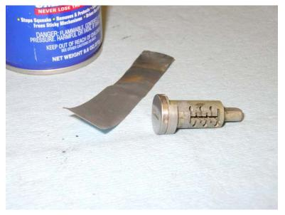
You can clean up the inside of the lock cylinder, the outside of the plug, and the slots where the wafers go with some 600-grit sandpaper wetted with WD-40.
